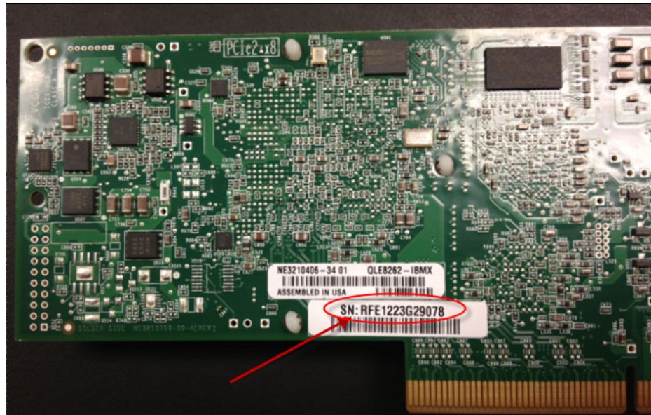
Figure 2-17 Physical inspection example of a QLogic card that shows the serial number
